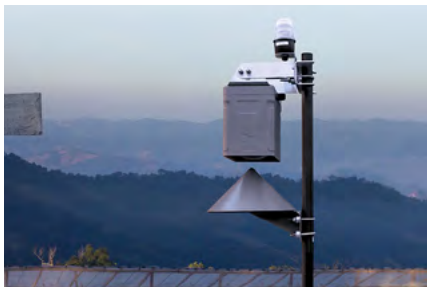
SFERIC SIREN AUTOMATED LIGHTNING ALERTING SYSTEM
