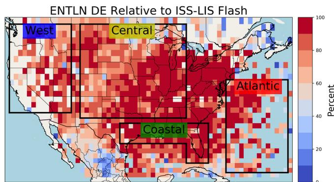
Relative to the Lightning Imaging Sensor aboard the International space station (ISS-LIS), ENTLN has a relatively constant detection efficiency throughout all four regions analyzed in this study.
